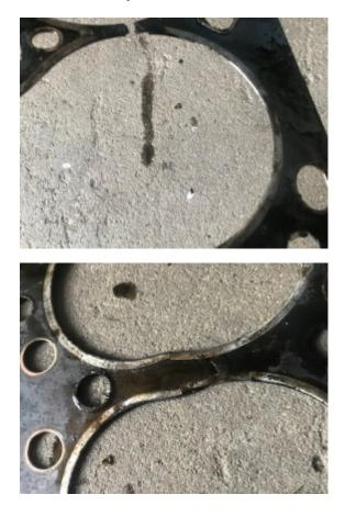
The cylinder head and the cylinder block Appear to have "fret " marks on the surface as if the head was moving. How should I determine if the cylinder liners
