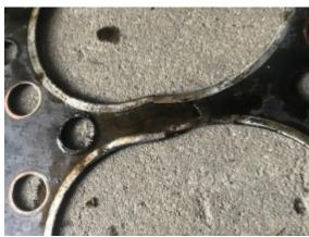
The cylinder head and the cylinder block Appear to have "fret " marks on the surface as if the head was moving. How should I determine if the cylinder liners
